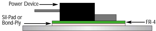
Mid Power Application with Bond-Ply
