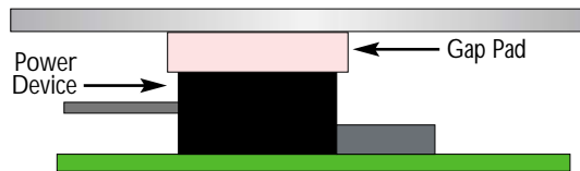
Lower Power Application with Gap Pad
